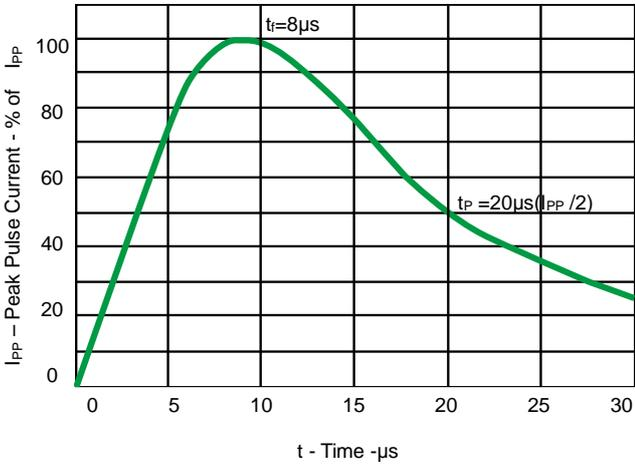
Fig 1. Pulse Waveform
