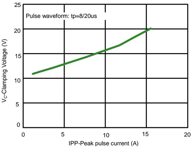
Fig 3. Clamping voltage vs. Peak pulse current
